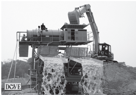
SUPERMINER-III DS (FEEDING WITH EXCAVATOR)
